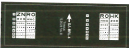
SA-BRL-4 — Visual Acuity Results calibrated at 20/20, 20/30, 20/40, 20/50, 20/70, 20/100, and 20/200. Tests can be administered binocularly or with either eye occluded.
