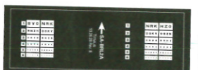
SA-BRL-2A — Visual Acuity Results calibrated at 20/20, 20/30, 20/40, 20/50, 20/70, and 20/100. Tests can be administered binocularly or with either eye occluded.
