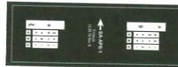
SA-APS-1 Allen Picture Test Line 1 — Binocularity — Tests performance of both eyes together. Lines 2, 3, 4 — Acuity — Right and Left Eye Calibrated at 20/30, 20/40 and 20/50.
